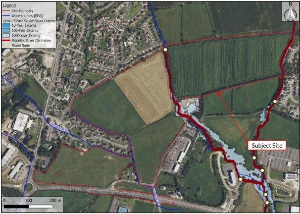
Figure 3-5 North Western CFRAM Current Fluvial Flood Extents
