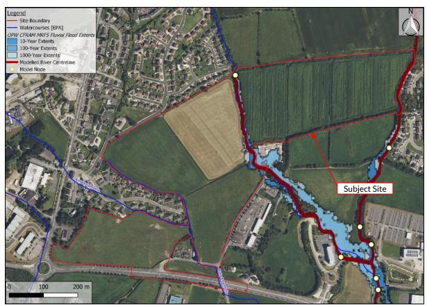
Figure 3-6 North Western CFRAM MRFS Fluvial Flood Extents
